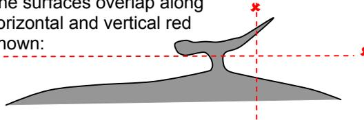
*Discussion point: Freedom to have overlapping surfaces in one plane, say the vertical, would allow some scope for the cars to look different. This would produce some interesting developments over time and allows perhaps more scope for the integration of cooling vents. It would still severely limit the scope for significant performance gains and avenues for experimentation.*
