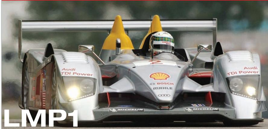
Features some of the most technically sophisticated race cars in the world, the top Le Mans Prototype (LMP) division is LMP1 - purpose-built racing machines such as the diesel-powered Audi R10 TDI, Creation CA06, Lola B06/10 and Zytek 06S among others. These ultra-engineered racing cars produce between 600-700 horsepower, have a minimum weight of 925 kilograms (approximately 2,040 pounds), can accelerate from 0-100 mph in three (3) seconds and reach top speeds in excess of 200 mph.
