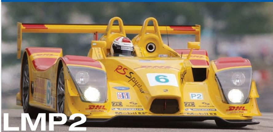
The smaller purpose-built race cars comprise the LMP2 class, including the Porsche RS Spyder, Lola B05/40, Acura-powered Lolas and Courages, Mazda-powered Lola and Radical SR9. Capable of reaching speeds of 180-200 mph, these highly sophisticated race cars produce between 500-550 horsepower and have a minimum weight of 775 kilograms (approximately 1,708 pounds).
