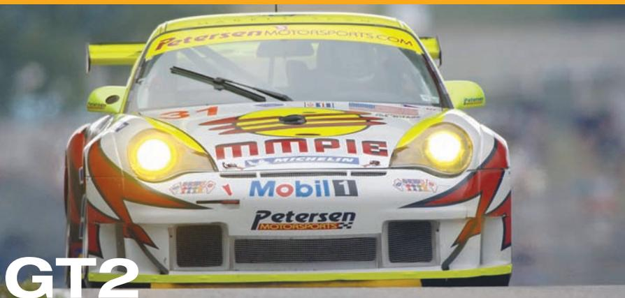
The production-based, moderately modified two-wheel drive race cars comprise the GT2 class - Ferrari 430 GT Berlinetta, Panoz Esperante GTLM and Porsche 911 GT3 RSR. With top speeds of up to 180 mph, these elite GTs produce between 450-500 horsepower and have a minimum weight of 1,125 kilograms (2,480 pounds).
