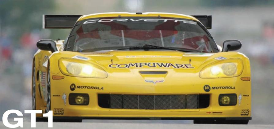
The top class in the Grand Touring (GT) division is GT1 featuring production-based two-wheel drive race cars such as the Corvette C6.R, Aston Martin DBR9 and Saleen S7R. Reaching speeds of 180-195 mph, these highly modified racing GTs produce between 600-650 horsepower and have a minimum weight of 1,125 kilograms (approximately 2,480 pounds).
